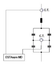
Within the bridge circuit, the phase position of the unbalance current L1, L2 and L3 in relation to the reference current is 0, +120, or +240 degrees. The ESTAsym® MD can reveal the fault phase and the bridge circuit branch in which the faulty capacitor unit is located.
