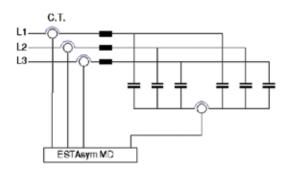
The double star circuit generates a sum current the size and phase of which result from the three unbalance currents. Using the reference current, the ESTAsym® MD can analyze the sum current into the three unbalanced currents. Each change of the sum current can take place only in the same phase of the capacitor current. Thus the ESTAsym® MD can reveal the partial path in which the defective capacitor unit is located. This means that only 1/6 of the capacitors need to be checked.
